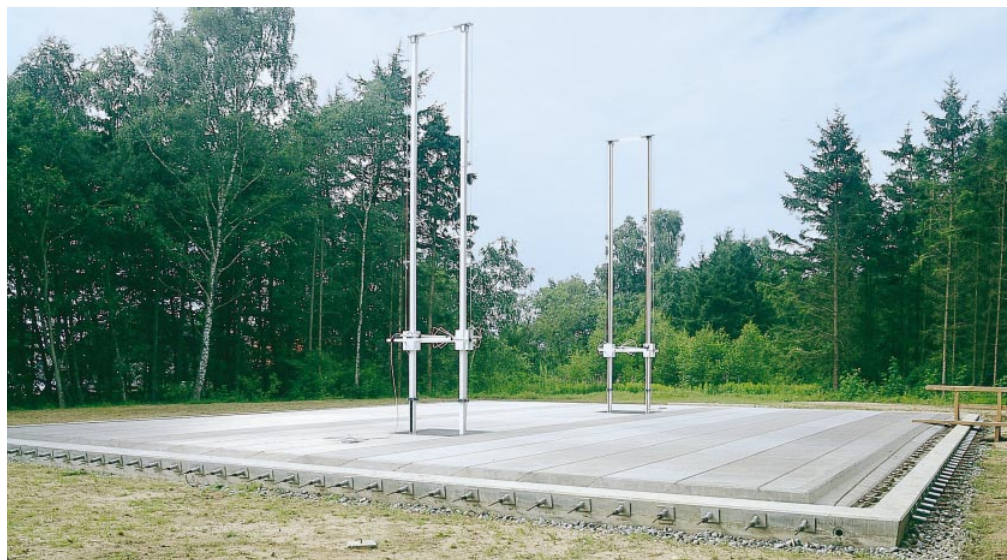
FIG 1 Open-area antenna test site of BAPT in Itzehoe with its two 8 m high antenna rigs
