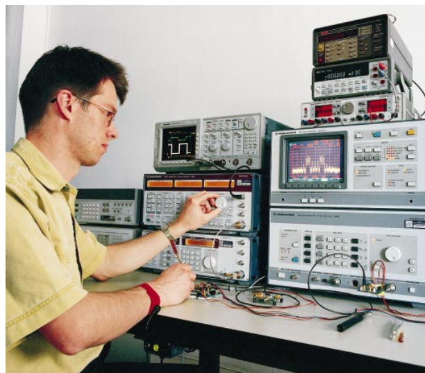
FIG 2 Test setup with EMI Test Receiver ESMI for BER measurement at Thesys Microelectronics Photo: Thesys GmbH
