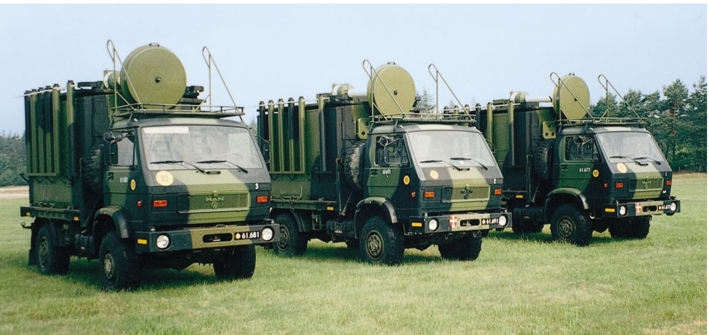
FIG 1 DAISY transport vehicles with shelters and folded-down VHF-UHF DF antenna from Rohde & Schwarz
