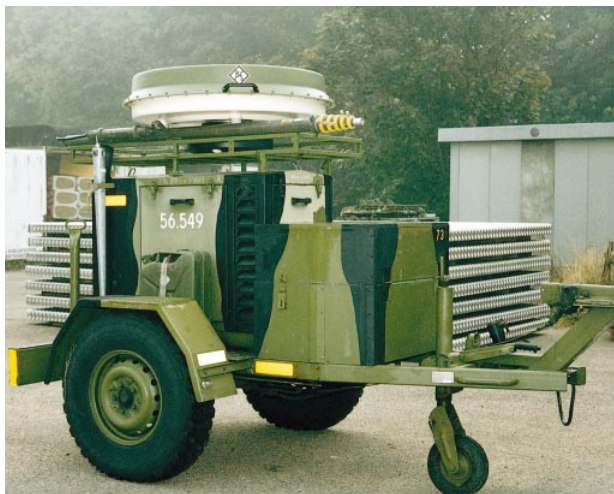
FIG 2 Trailer for transporting power generator of DF system and HF DF antenna Photos: Madsen
